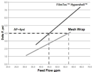
Pressure Drop versus Feed Flow for Mesh wrap and FilmTec™ Hypershell™ 8038 elements. FilmTec™ Hypershell™ has less exterior bypassing and requires approximately 30% less flow than mesh wrap for an equivalent pressure drop.
