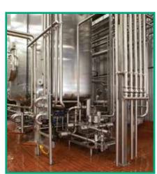
Your product quality is ensured because all product valves can be lifted during cleaning (CIP), leaving no potentially contaminating residue behind. Therma-Surge can be installed into your existing sterilization line or as part of a complete system.
