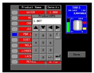
Operator or Admin Access – if you are password entered into this access level, you can edit the product name or add a new product designation to the list (and enter a specific gravity value). Simply touch the existing text or touch an unused position to launch the on screen entry keypad.
