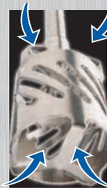
**3.** Centrifugal pressure forces material to the periphery of the stator where it is subjected to further mechanical shear as material passes through the sharpened edges of the expanded slots in the stator.
