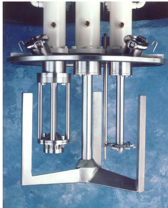
Triple-Shaft Mixer composed of a high shear rotor/stator (left), three-wing anchor (center shaft), and a disc-style disperser blade (right). All three agitators are independently- driven.
