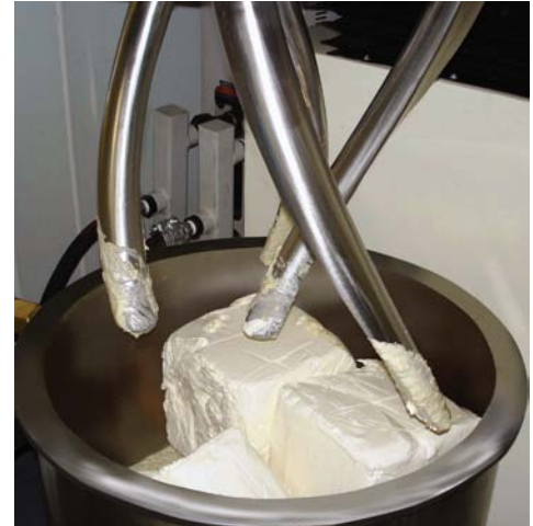
The trailing slope and helical design of the HV blades work well in this specialty cheese application, creating five times the product in half the time of a conventional mixer.
