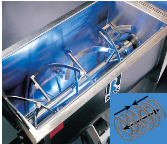
Anatomy of a ribbon blender: The inner and outer ribbons are pitched to move material axially, in opposing directions, and also radially. This combination promotes fast mixing.
