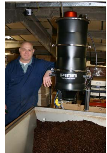
Fresh coffee beans are transported through a vacuum conveyor.
