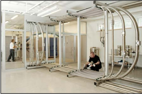
PIAB's testing facility allows customers to test powder, granule or fluid samples. Testing ensures the vacuum cycle time and energy consumption are effective.
