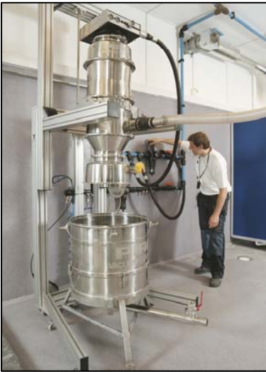
Stainless steel C-Series conveyors are ideal for conveying starches, powders and other dry ingredients. Powered by pneumatically driven vacuum pumps, these systems safely and quietly transport up to 10-15 tons/hour of material.
