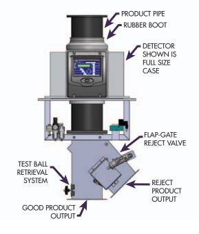
Also... a metal detector can be configured to operate in 'Pipeline' mode, where the product is generally pumped through the system (shown below) and contamination is diverted away from the product flow through the 'Reject Valve'.
