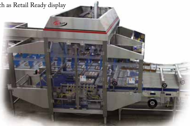
Delkor's Flex Loader 1000 series loads product up 700 containers per minute.
