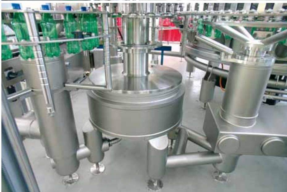
machine design extremely simple and therefore means a very high standard of hygiene: all the pneumatic connections have been completely eliminated
