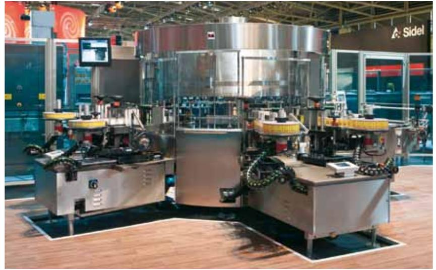
**8** The servomotor-driven SL 90 labeler for both cold-glued paper labels and self-adhesive transparent labels.
