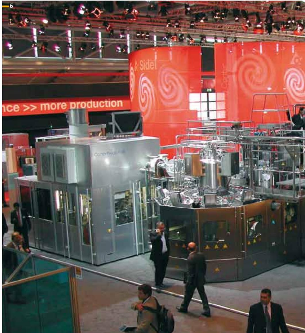
6 Combi Predis FMa, the first aseptic Combi, which enables the bottling of UHT milk in PET, with dry decontamination of preforms.
