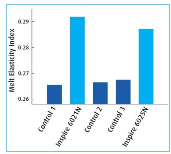
Higher melt strength will translate to more stable drawing during the thermoforming process and also result in a more uniform wall thickness distribution in the final part.
