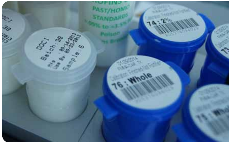
Milk calibrations standards from DQCI laboratories, preheated on 40 C All MPA are pre-calibrated based on DQCI samples
