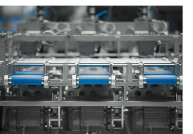
wrap around case packer for horizontal and vertical packing patterns
