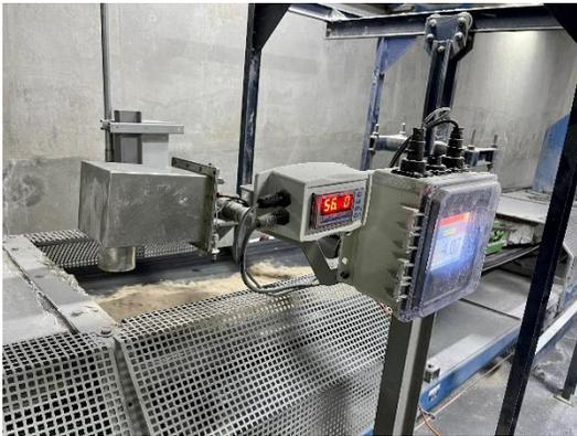
Optimizing the manufacturing process to include a moisture measurement and control system improves product quality and production efficiency and reduces the amount of dust and build-up created. Small variations in moisture content can result in clumping, affecting the quality and consistencies in the production; absence of moisture can result in excess dust. Non-contact moisture detection can provide real-time accurate data to help line personnel to properly control and eliminate common issues.
