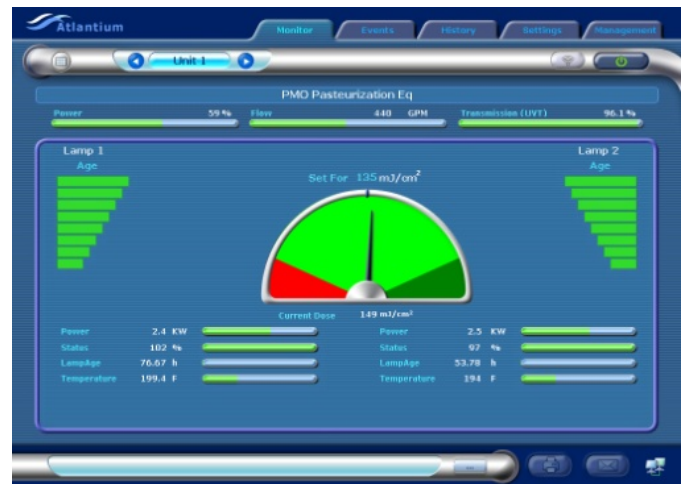
Figure 3: Monitor shows status of critical parameters in real-time, including actual dose being delivered.
