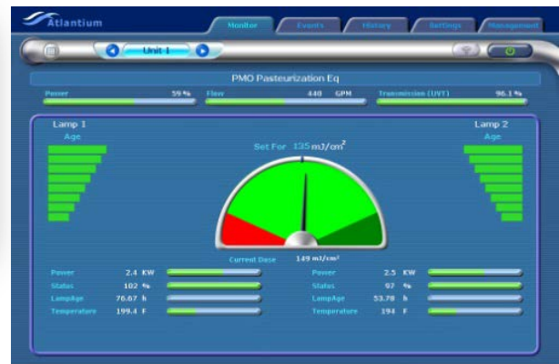
Fig 3: Monitor shows status of critical parameters in real-time, including actual dose being delivered.
