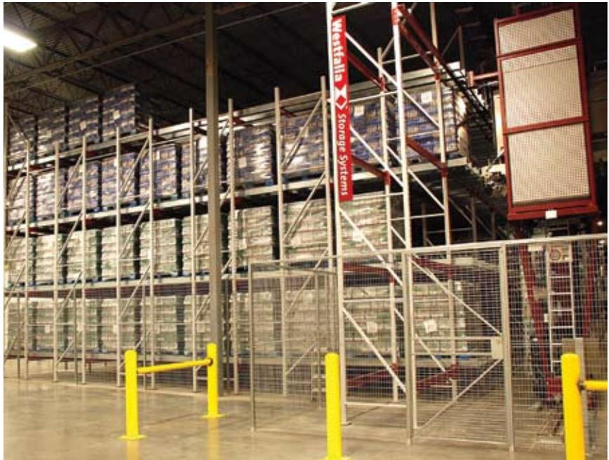
directly to the shipping dock via Westfalia's unique Drawbridge Conveyor, which was designed specifically for this project. The Drawbridge Conveyor either lays across the crane aisle for pallets to travel directly to the shipping dock, or it lifts straight up for the S/RM to move through the aisle. The lifting operation takes only seconds.
