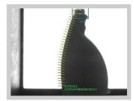
Checking sealing surface for molding flash
