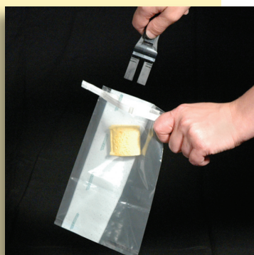
Return to bag, release sponge into bag, twirl bag closed and send to lab for analysis.
