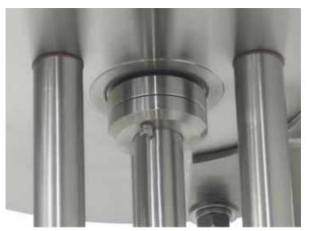
The C-Type sanitary mechanical seal enhances the cleanability of the machine by eliminating all potential product trap areas and allowing direct CIP spray to the mechanical seal assembly.
