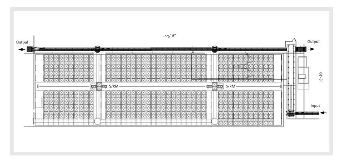
Automating the product flow -- from palletizing to shrink-wrapping to conveyors and into the AS/RS -- provided seamless warehousing and major labor savings for Blue Bell. When it comes time to pick the product for orders, the WMS calls for the product and the AS/RS delivers it to the conveyor.
