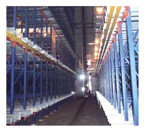
To streamline Blue Bell's production and storage facility, the project's sec ond phase included installing an Automated Storage and Retrieval System (AS/RS) consisting of two Storage Retrieval Machines (S/RM) operating in one aisle. This design provides redundancy should an SRM require maintenance. For this particular operation, the individual SRM holds 2 pallets, and has its own designated "working area" and safety zone.
