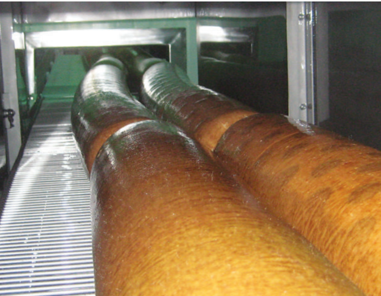
(LEFT) Step 1: Logs are delivered to the slicing room through a spray cabinet where the entire product surface is treated with antimicrobial spray at a specified dwell time. (RIGHT) Step 2: An antimicrobial solution is also applied at the blade during the slicing operation.
