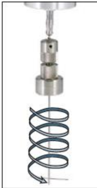
Figure 2: T-bar Type Spindle for Viscosity Testing on Cottage Cheese
