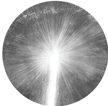
Pictured left: THE IMPINGEMENT ZONE. Concentrated stream of a Gamajet and the tangential force radiating from the point of impact.
