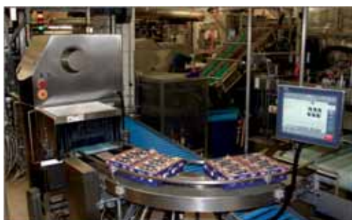
X-ray scanner SC 5000 with separate display - individually adjustable and easy to operate
